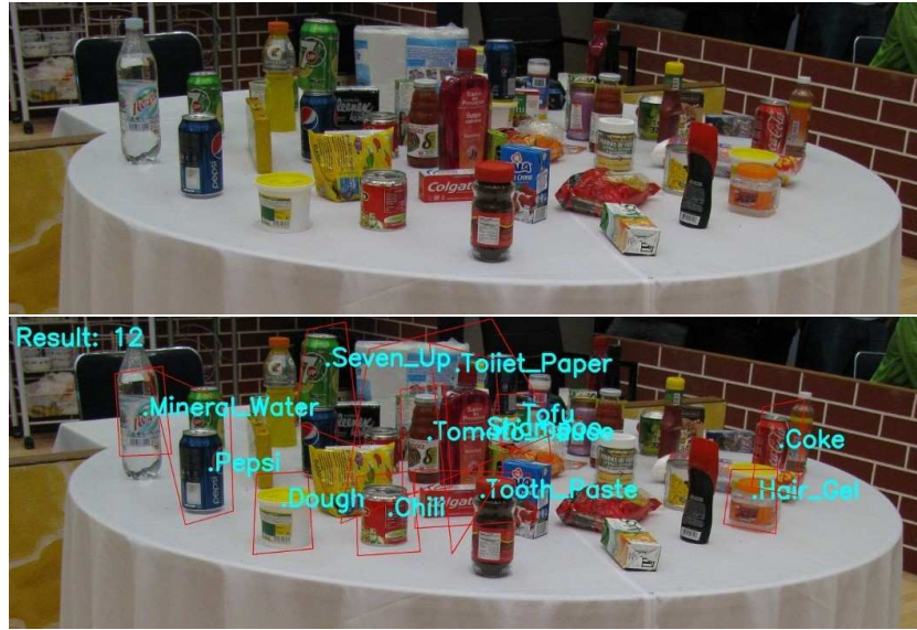
Fig. 9. The input image for object recognition as acquired by our robot during the Technical Challenge of the RoboCup (top). Object recognition results with 12 correctly identified objects (bottom). During training and recognition an image resolution of 8 MP was used.
